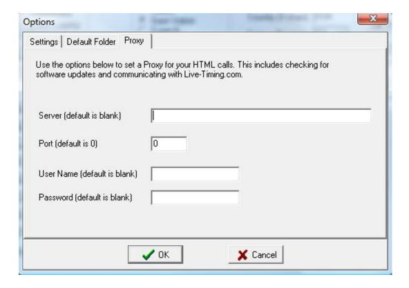
Some networks at resorts require web interfaces be managed through a proxy. This page is used to set the values for the proxy. Contact your network administrator for the correct values to use.
